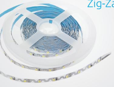
The Zig-Zag LED Reel is an adaptable and flexible lighting solution. There are 60 LEDs per metre on a 5-metre roll with the ability to cut every 3 LEDs. It provides even illumination for a wide range of signage applications including; built up 3D letters, halo effect signage and flat shapes.
